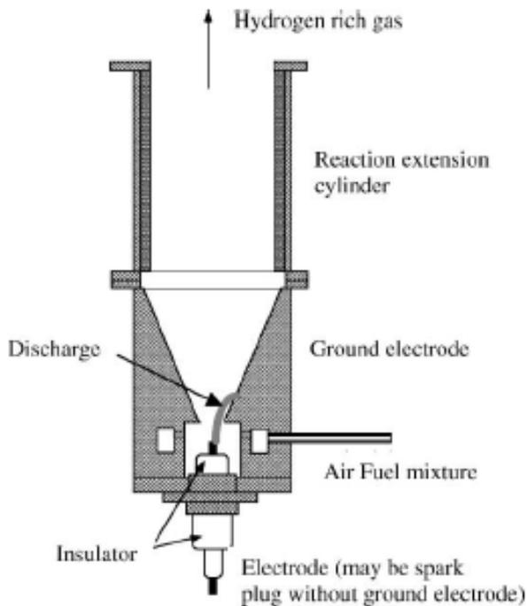
Figure 10: Low current plasmatron fuel reformer [14]
