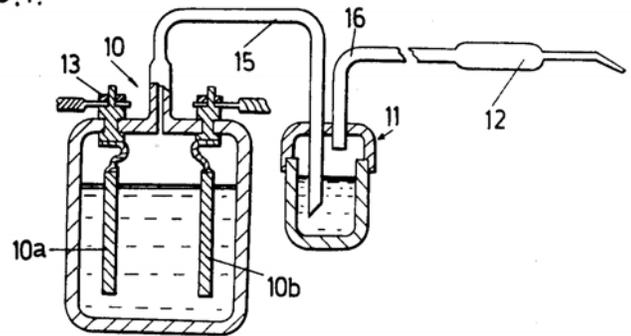
Figure 13: Yull Brown's electrolysis unit from US Patent: 4,081,656 [18]
