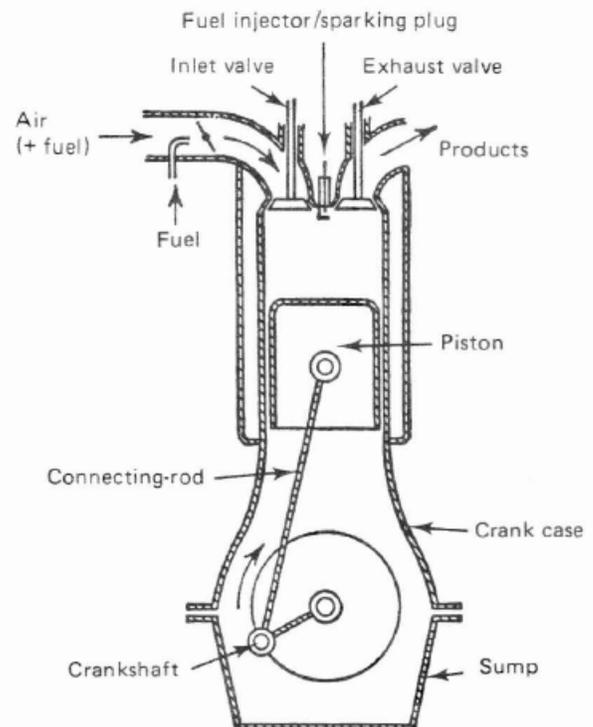
Figure 1: Four Stroke Internal Combustion Engine [1]
