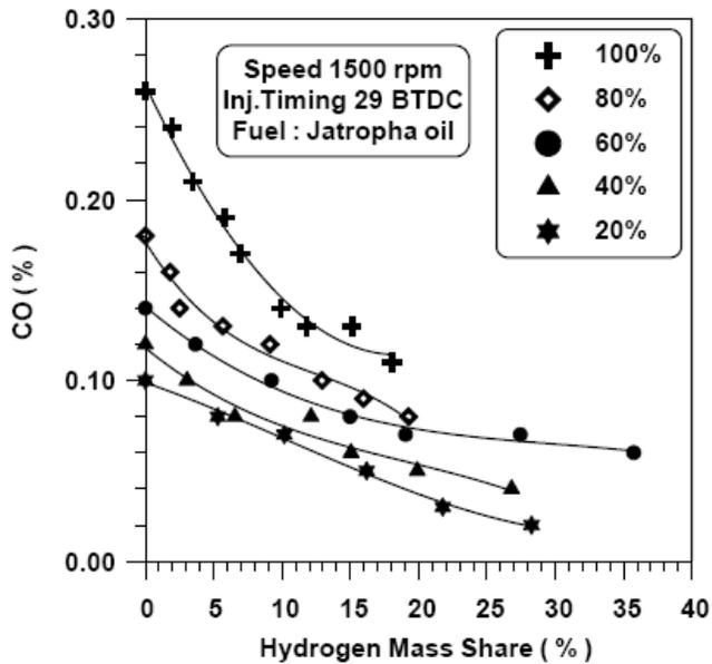
Figure 6: Effect of H<sub>2</sub> addition on jatropha oil combustion CO emissions [6]
