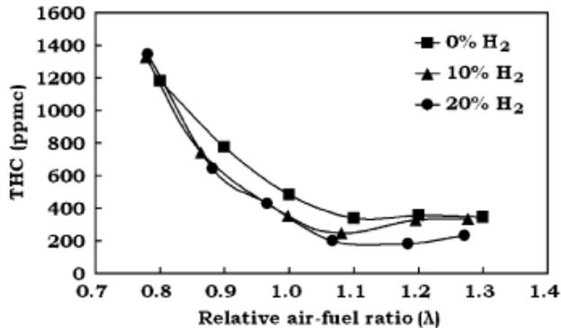
Figure 7: Effect of H<sub>2</sub> addition on natural gas combustion hydrocarbon emissions [8]
